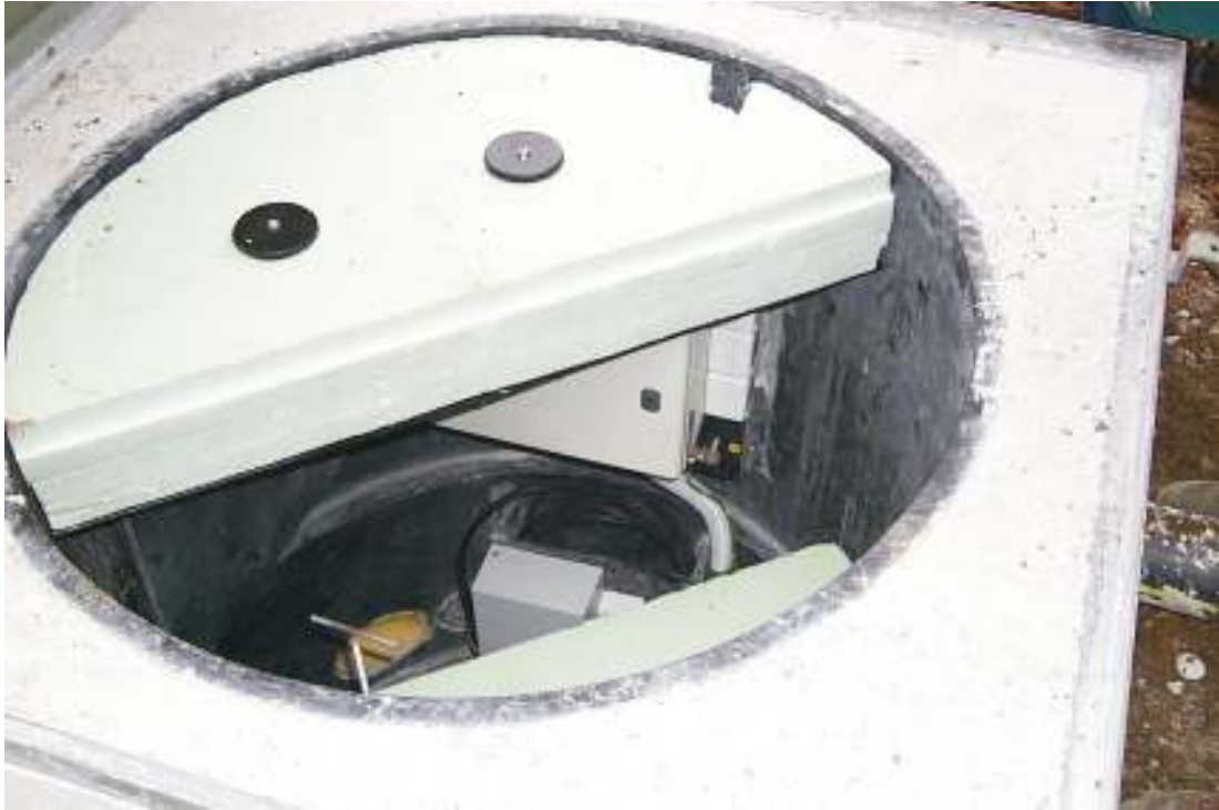
Slika 15. Pogled v jašek z merilnimi instrumenti. Senzor je postavljen v vrtino pod jaškom. Figure 15. A view of the shaft's interior with measuring instruments. The sensor is placed into the borehole below the shaft.
