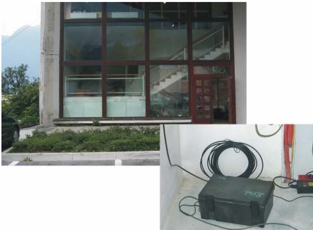
Slika 4. V Bovcu je akceleroграф Etna nameščen v pritličju knjižnice. Figure 4. Accelerograph Etna is placed in the basement of the public library in Bovec.
