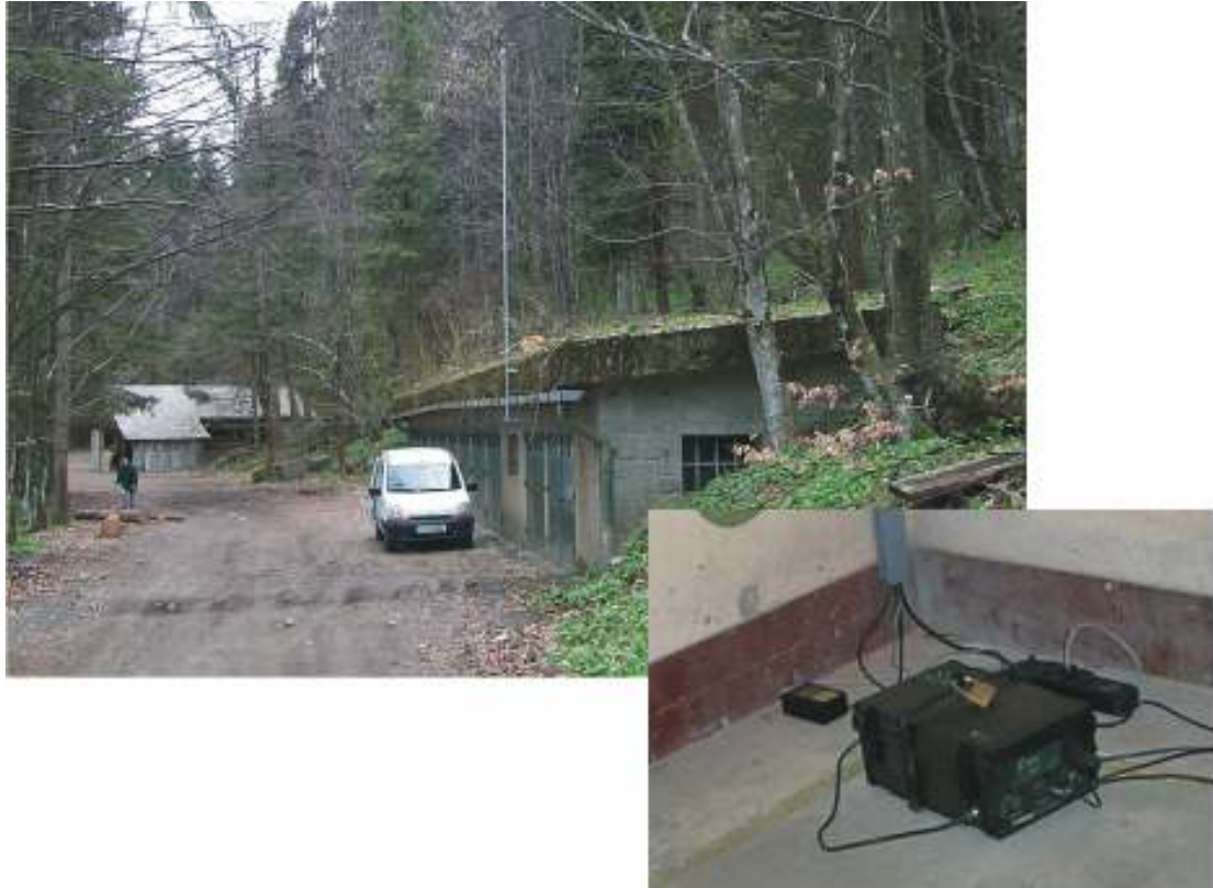
Slika 6. Objekt v Gotenici, v katerem je nameščen akceleroграф Etna. Figure 6. Structure in Gotenica, where accelerograph Etna is placed.
