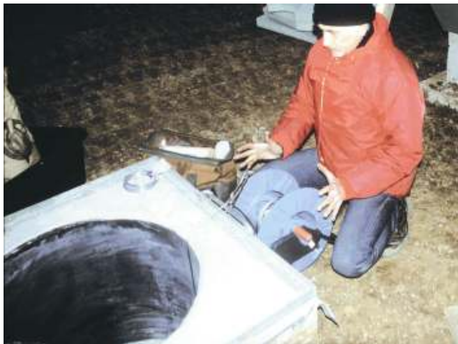
Slika 3. Spuščanje seizmometra v vrtino Figure 3. Lowering of the seismometer in the borehole
