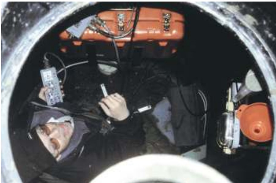
Slika 4. Kontrola lege seizmometra s HCU enoto Figure 4. The control of the seismometer's position with an HCU unit
