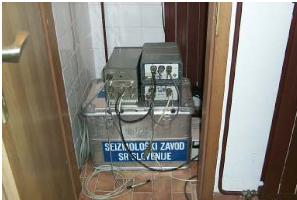
Slika 10. Prenosna opazovalnica s seizmometrom v kleti gasilskega doma v Gaberkah Figure 10. The temporary station with a seismometer in the cellar of the Firebrigade station in Gaberke
